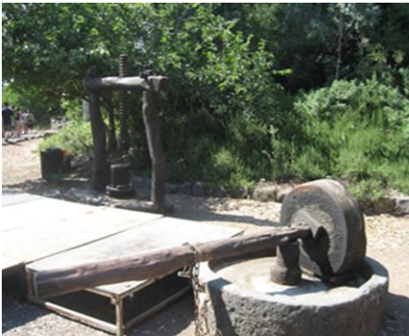
Olive Grinder used to grind olives including seeds. An olive press is in the back used to press the olive oil out of the crushed olives and seeds from the grinder.
